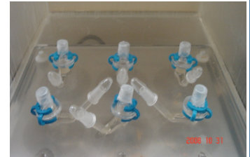
Figure 1 - Support with Franz diffusion cells (n=6) in a heat water bath (32°C)
