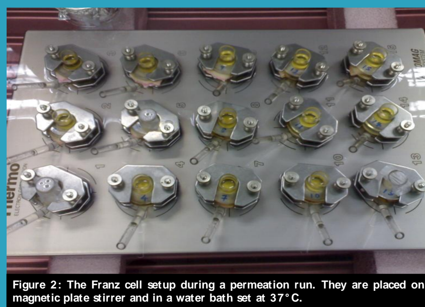
Figure 1: Upright Franz Diffusion. The skin pieces were mounted in between the donor and the receptor phase.
